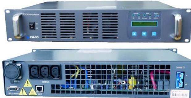
CSI series inverters with integrated static switch supplies uninterrupted, highly efficient and stable single phase AC sine wave voltage from a battery bank. The magazine design can be easily installed into 19 inch cabinets, and designed for use in telecom, communication, finance, utilities, transportation, military and other fields.
