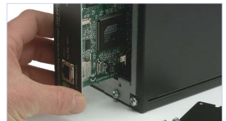
APC accessory cards can be inserted into the built-in SmartSlot to allow monitoring of power conditions. The Smart-UPS RT 5000, 7500, and 10,000 units ship bundled with the Web/SNMP Management Card
