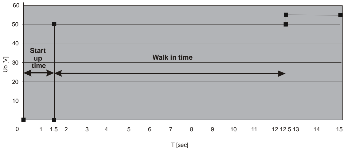
Figure 4-4 Start up behaviour typ.: Output Voltage vs. Time
